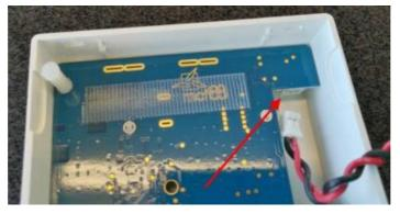
• Connect the new batteries and put them in place (replace the tape if needed):
