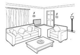
The device must be placed where the LoRaWAN signal coverage is good (SF = 7 optimal, SF = 12 weak). The sensor must be installed vertically on a wall at about 1.5mt height. It must be at least 30cm away from metal objects, and 1mt away from electronic devices.
